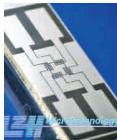
Full bridge strain sensor.
