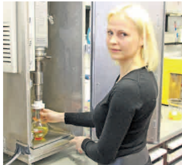
Dr. Andreeva demonstrates the procedure of sonication of solid particles in an aqueous suspension by using the UIP1000hd horn ultrasound device.
